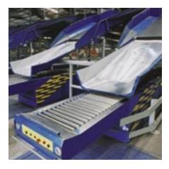
The operator can extend the conveyor into confined spaces whilst delivering cartons, sacks, bags, parcels, tyres etc at constant speeds.
