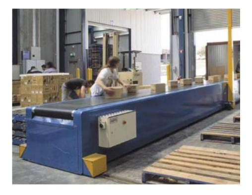
back and forth. The adoption of loose loading / unloading eliminates all waiting time. A constant stream of product is delivered to the fingertips of the operator.
